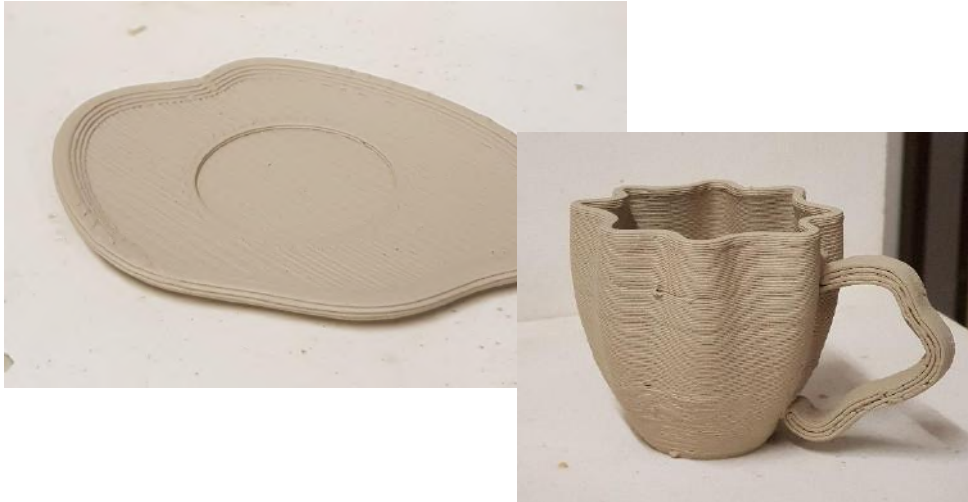
Image 13.14. Printed plate and cup, left to dry
