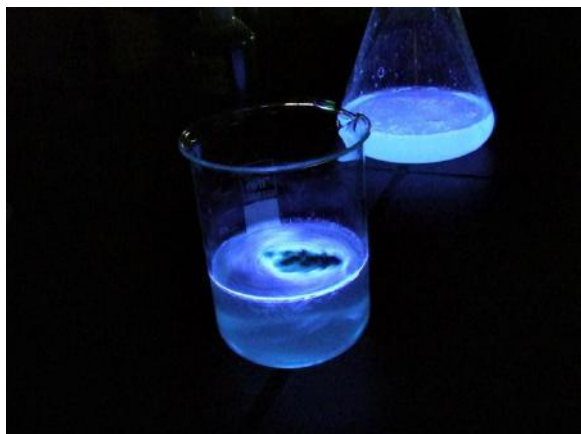
Figure 1. Luminol and Hemoglobin. Luminol glows in an alkali solution when added Hemoglobin and \text{H}_2\text{O}_2 [10].
