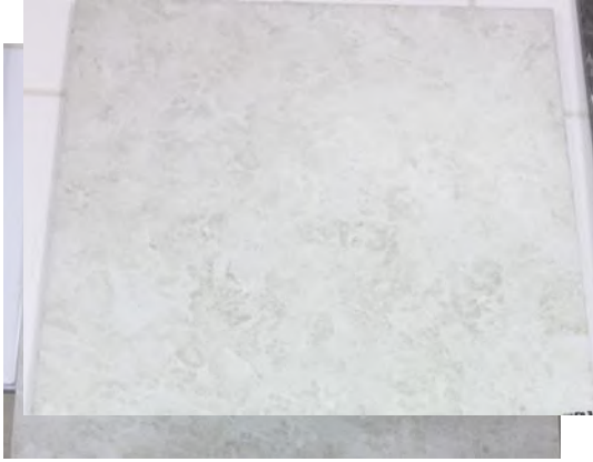
Figure 5. Engobe+Glaze+Digital printing with light colored image
