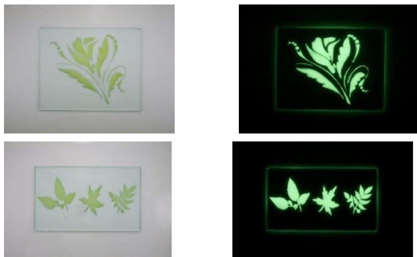
Figure 26. Flat glass with yellowish–green phosphorescence pigment–epoxy resin mixture and decor application [42, 44, 47, 57].
