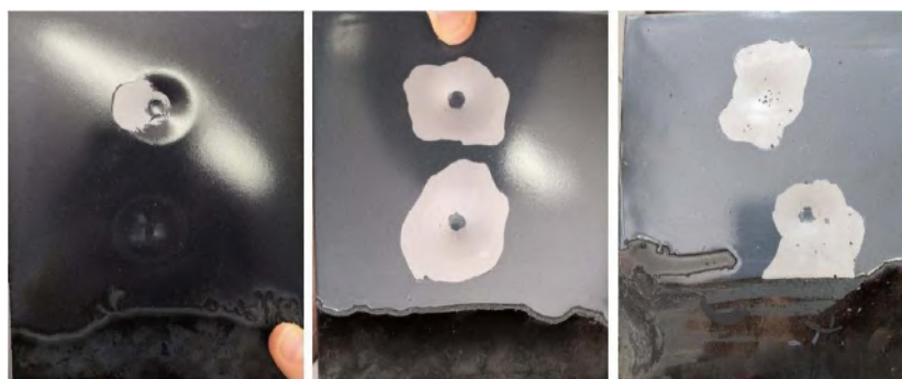
Figure 3. Samples images after impact test: GLFLY7 IND (a); GLFLY7 LAB (b); GLFLY0 (c).
