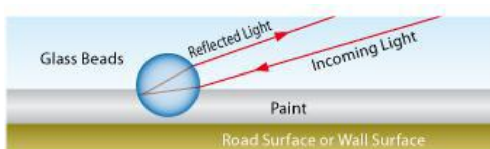
Figure 12. Phosphorescent glass beads have retro-reflectivity enabling high visibility and ornamental effect. Retro-reflection model of glass beads [27].
