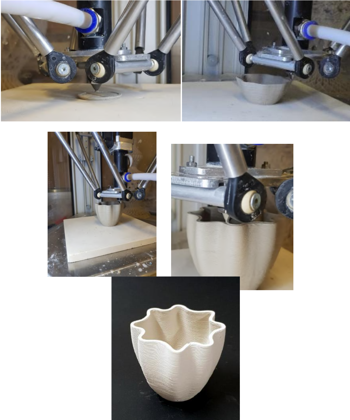
image 8.9.10.11.12. Printing layer by layer from base to top
